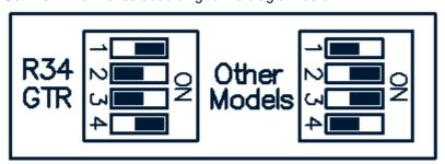
Some GTS/GTR transmissions use a Throttle Position Out signal from the ECU for correct control. There are two scale options for this: '1:1' and '2:3'. The usual position is '2:3', however if you find your transmission produces fault codes try the '1:1' jumper option
